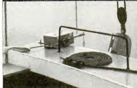
Small box attached to rail houses unit which rings bell in cabin if suspended lead-line strikes bottom
